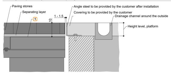
1 Sealing of the pit (see "Detail of building configuration - pit sealing", page 8)
